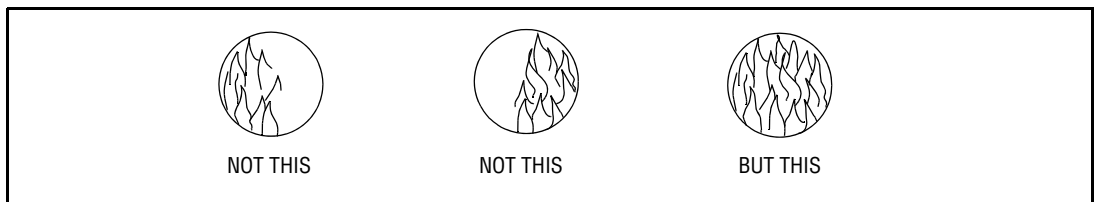
FIGURE 6. FLAME MUST COMPLETELY COVER SIGHT OPENING
