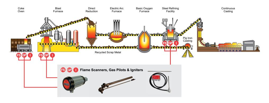
Ultraviolet (UV), Infrared (IR), Dual Sensor (UV & IR) Flame Scanners along with High-Energy Spark Igniters (HESI) and Gas Pilots.
